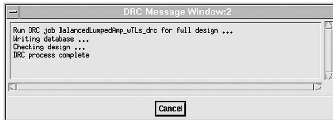
Figure B-3. Message that appears after the DRC has been run.
